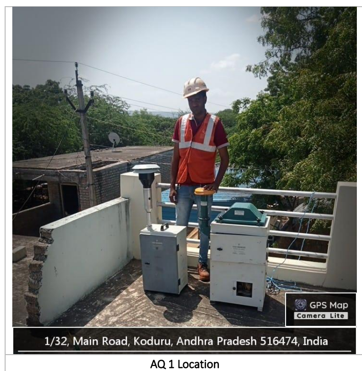
Figure 4:6 Ambient air quality test and monitoring conducted in Study Area
